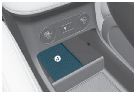
[A] : Wireless Charging Pad (In-vehicle Authentication Pad)
