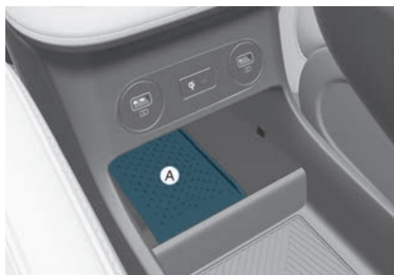
[A] : Wireless Charging Pad (In-vehicle Authentication Pad)
