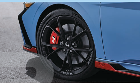
19” forged wheels and 14.2” front brake rotors
