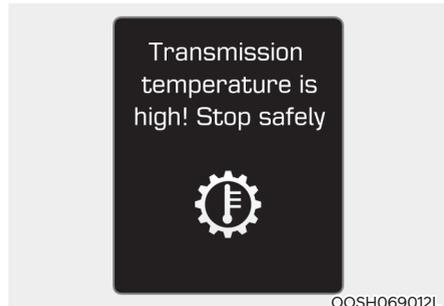
Repeated stop-and-go launches on steep grades, sudden take off or acceleration, or other harsh driving conditions may increase the clutch and transmission temperature.
