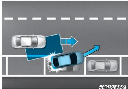
When you are driving forward out of a parking space, if Blind-Spot Collision-Avoidance Assist judges that there is a collision risk with an approaching vehicle in the blind spot, Blind-Spot Collision-Avoidance Assist will help avoid collision by applying the brake.
