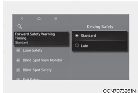
With the engine on, select **User Settings > Driver Assistance > Driving Safety > Forward Safety Warning Timing** from the settings menu in the instrument cluster or **Setup > Vehicle > Driver Assistance > Driving Safety > Forward Safety Warning Timing** settings menu in the infotainment system to change the initial warning activation time for Forward Collision-Avoidance Assist. The warning time can be set to either Normal or Late.
