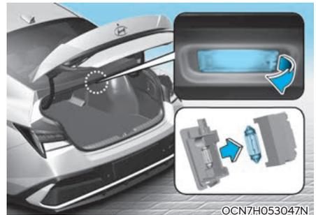
1. Using a flat-blade screwdriver gently pry the assembly from the lamp housing.
