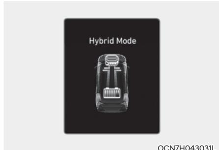
This mode displays the engine status for each area, such as the power transmission status of the hybrid system according to the driving condition, starting and accelerating, constant speed driving, and deceleration.
