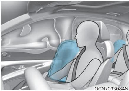
The side airbags are designed to deploy only during certain side impact collisions, depending on the crash severity. The side and curtain airbags on both sides of the vehicle may deploy if a rollover or possible rollover is detected. For vehicles equipped with a rollover sensor the side airbags and pre-tensioners on both sides of the vehicle may deploy if a rollover or possible rollover is detected. However, the side airbags are not designed to deploy in all side impact or rollover situations.
