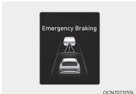
To warn the driver that emergency braking will be assisted, Forward Safety warning light (🚨) blinking, the 'Emergency braking' warning message will appear on the instrument cluster, an audible warning will sound.
