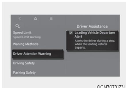
With the engine on, select or deselect **User Settings > Driver Assistance > Driver Attention Warning** from the settings menu in the instrument cluster or **Settings > Vehicle > Driver Assistance > Driver Attention Warning** from the settings menu in the infotainment system to set whether to use the function.
