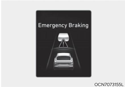
To warn the driver that emergency braking will be assisted, the 'Emergency Braking' warning message will appear on the cluster and an audible warning will sound.
