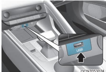
The USB port can be used while the engine is running.
