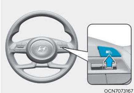
Press the Driving Assist (Ⓜ) button to turn off Cruise Control. The Cruise (ⓂCRUISE) indicator light goes off.
