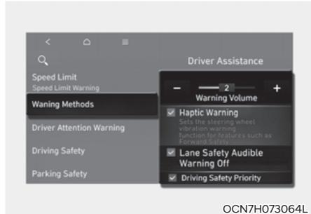
The Warning Methods can be set with the vehicle on. Select **User Settings > Driver Assistance > Warning Methods** from the settings menu in the instrument cluster or **Setup > Vehicle > Driver Assistance > Warning Methods** from the settings menu in the infotainment system to change the following settings:
