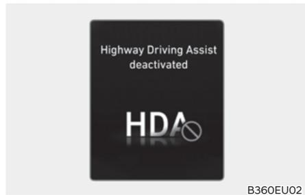
If the driver still does not have their hands on the steering wheel after the hands-off warning, the "Highway Driving Assist deactivated" warning message may appear and Highway Driving Assist is automatically canceled.
