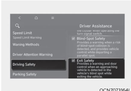
With the engine on, select **User settings > Driver Assistance > Driving Safety > Exit Safety** from the settings menu in the instrument cluster or **Settings > Vehicle > Driver Assistance > Driving Safety > Exit Safety** from the Settings menu in the infotainment system to turn on Safe Exit Warning and deselect to turn off the function.
