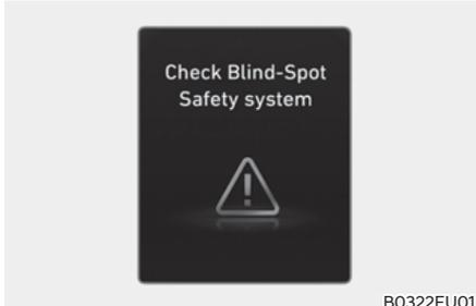
When Safe Exit Warning is not working properly, the "Check Blind-Spot Safety system" warning message will appear on the instrument cluster for several seconds, and the master (⚠) warning light will appear on the instrument cluster. Have the vehicle inspected by an authorized HYUNDAI dealer.
