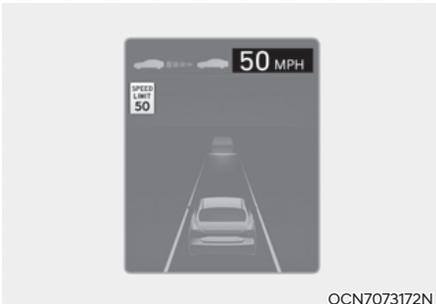
Manual Speed Limit Assist or Smart Cruise Control assists the vehicle to adjust its speed according to the speed limit. When the cruising speed is set as same as the speed limit, the vehicle automatically adjusts its speed if the speed limit changes. The function operates on the road which has a speed limit of 45 mph (70 km/h) or higher. When the function is active, the cruising speed on the instrument cluster appears in green.
