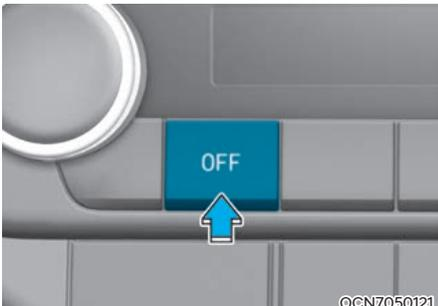
Push the OFF button of the front to turn off the air climate control system. However, you can still operate the mode and air intake buttons as long as the ignition switch is in the ON position.
