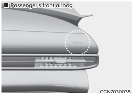
The purpose of the SRS is to provide the vehicle's driver and front passengers with additional protection than that offered by the seat belt system alone. The SRS uses sensors to gather information about the driver's and front passenger's seat belt usage and impact severity.
