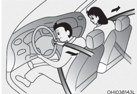
Your vehicle is equipped with driver's and front passenger's and rear passengers Pre-tensioner Seat Belts (Retractor Pre-tensioner). The purpose of the pre-tensioner is to make sure the seat belts fit tightly against the occupant's body in certain frontal or side collision(s).
