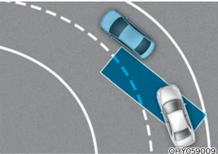
Blind-Spot Collision-Avoidance Assist may not operate properly when driving on a curved road. Blind-Spot Collision-Avoidance Assist may recognize a vehicle in the same lane. Always pay attention to road and driving conditions while driving.
