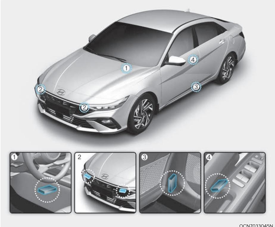
1. SRS control module/Rollover sensor
