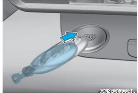
If the smart key battery is weak or the smart key does not work correctly, you can start the engine by pressing the Engine Start/Stop button with the smart key in the direction of the picture above.
