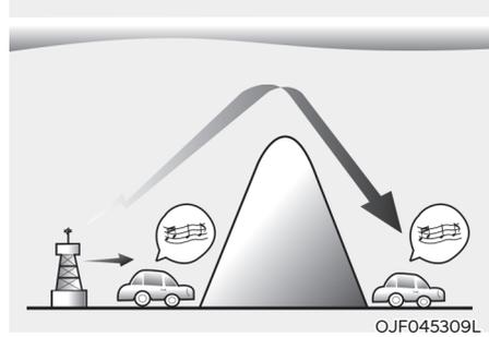
AM broadcasts can be received at greater distances than FM broadcasts. This is because AM radio waves are transmitted at low frequencies. These long, low frequency radio waves can follow the curvature of the earth rather than travelling straight out into the atmosphere. In addition, they curve around obstructions so that they can provide better signal coverage.
