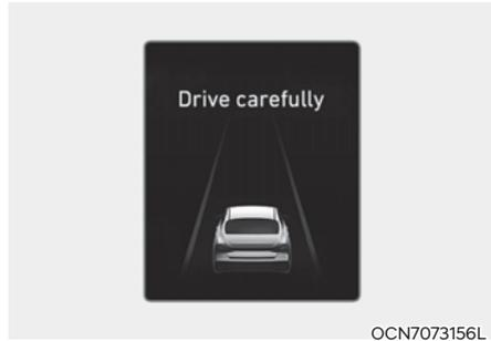
After your vehicle is stopped following an Emergency Braking event, the "Drive carefully" warning message may appear on the instrument cluster.
