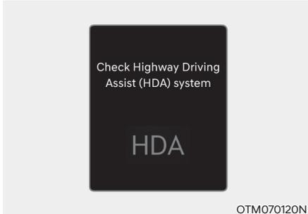
When Highway Driving Assist is not working properly, the 'Check Highway Driving Assist (HDA) system' warning message will appear, and the
