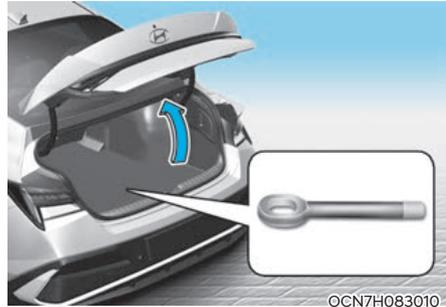
1. Open the trunk, and remove the towing hook from the tool case.
