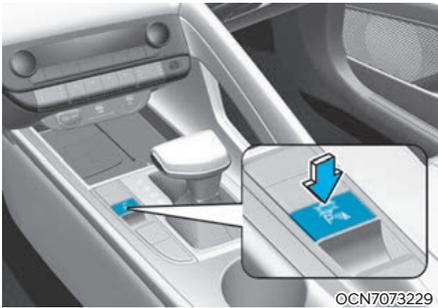
Press and hold the Parking Safety (P) button more than 2 seconds, to turn the Parking Collision-Avoidance Assist on or off.
