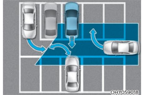
Rear Cross-Traffic Collision-Avoidance Assist may detect vehicles which are parking or pulling out near your vehicle (for example, a vehicle leaving beside your vehicle, a vehicle parking or pulling out in the rear area, a vehicle approaching your vehicle making a turn, etc.). If this occurs, the system may unnecessarily warn the driver and control the brake.
