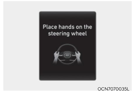
If the driver takes their hands off the steering wheel for several seconds, the 'Place hands on the steering wheel' warning message will appear on the cluster, and an audible warning will sound in stages.
