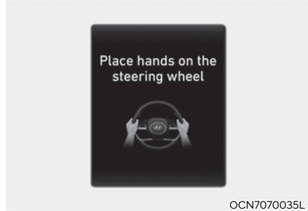
If the driver takes their hands off the steering wheel for several seconds, the 'Place hands on the steering wheel' warning message will appear and an audible warning will sound in stages. First stage : Warning message
