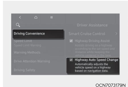
With the ignition switch ON, go to **Settings > Vehicle > Driver Assistance > Driving Convenience > Highway Auto Speed Change** from the Settings menu to turn on Navigation-based Smart Cruise Control and deselect to turn off the function.
