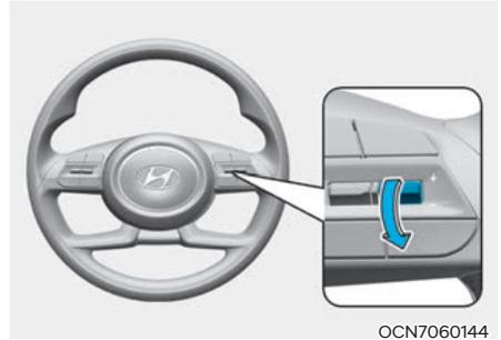
2. Push the + switch up or - switch down to change the set speed.
