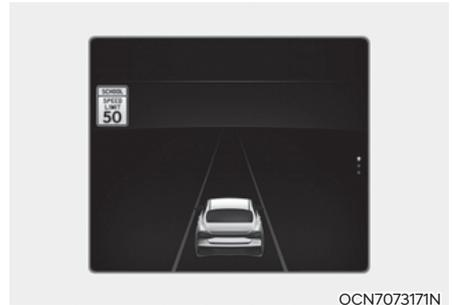
When driving at a speed higher than the displayed speed limit, the speed limit appears in red.
