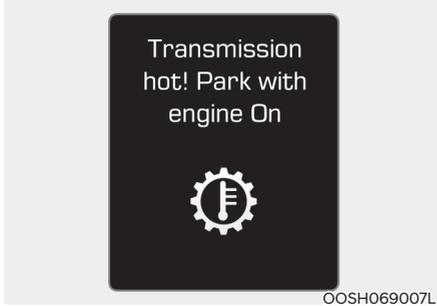
If you continue to drive with an overheated transmission, the above warning message appears, and the self-protection mode disables the clutch.
