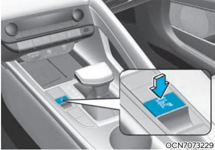
Press the Parking Safety (P) button to turn on Forward/Reverse Parking Distance Warning. Press the button again to turn off the function.
