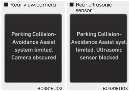
The 'Parking Collision-Avoidance Assist system limited. Camera obscured' or 'Parking Collision-Avoidance Assist syst. limited. Ultrasonic sensor blocked' warning message may appear on the instrument if:
