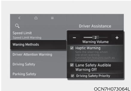
The Warning Methods can be set with the vehicle on. Select **User Settings > Driver Assistance > Warning Methods** from the settings menu in the instrument cluster or **Setup > Vehicle > Driver Assistance > Warning Methods** from the settings menu in the infotainment system to change the following settings:
