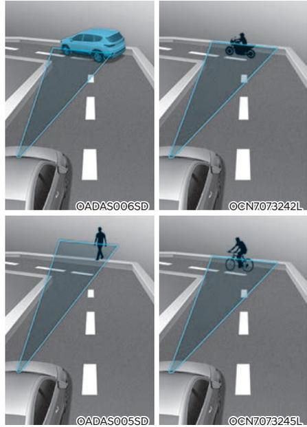
Forward Collision-Avoidance Assist may detect a vehicle, powered two-wheeler, pedestrian or a cyclist in the next lane or outside the lane when driving on a curved road.
