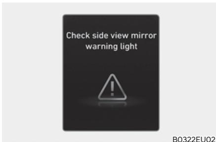
When the side view mirror warning light is not working properly, the "Check side view mirror warning light" warning message will appear on the instrument cluster for several seconds, and the master (⚠) warning light will illuminate on the instrument cluster. Have the vehicle inspected by an authorized HYUNDAI dealer.
