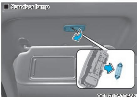
1. Using a flat-blade screwdriver, gently pry the lens or assembly from the interior lamp housing.
