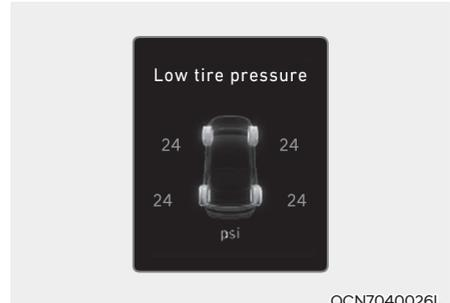
When the tire pressure monitoring system warning indicators are illuminated and a warning message displayed on the cluster display, one or more of your tires is significantly under-inflated. The Low Tire Pressure Position Telltale will indicate which tire is significantly underinflated by illuminating the corresponding position light.
