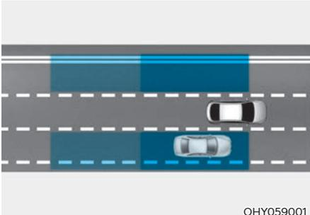
Blind-Spot Collision-Avoidance Assist helps detect and inform the driver that a vehicle is in the blind spot.
