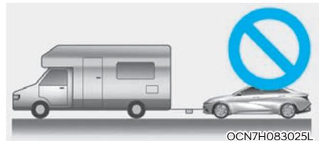
Otherwise, the transmission will be seriously damaged. Also, make sure not to tow the vehicle connecting it with other vehicles including camper vans.
