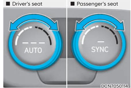
2. Turn the temperature control knob to set the desired temperature. If the temperature is set to the lowest setting (Lo), the air conditioning system will operate continuously.
