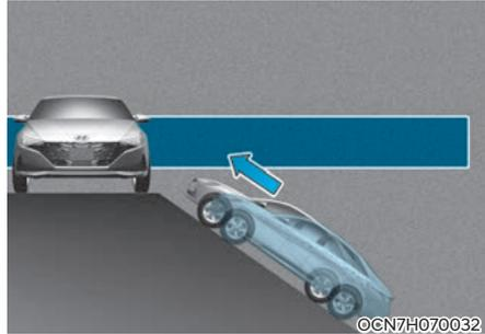
**Rear Cross-Traffic Collision-Avoidance Assist may be limited when the vehicle is on a uphill or downhill slope, or near it, and may not detect the vehicle approaching from the left or right. If this occurs, the system may not warn the driver or control the brakes when necessary.**
