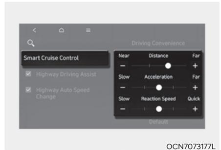
With the engine on, select **User settings > Driver Assistance > Smart Cruise Control** from the settings menu on the instrument cluster or **Settings > Vehicle > Driver Assistance > Driving Convenience > Smart Cruise Control** in the infotainment system to change Distance, Acceleration, Reaction Speed manually.
