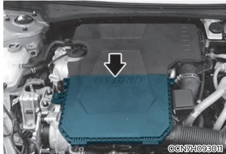
The air cleaner filter can be cleaned for inspection using compressed air. Do not attempt to wash or to rinse it, as water will damage the filter. If soiled, the air cleaner filter must be replaced.
