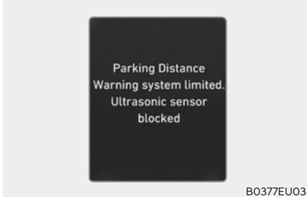
If this occurs the 'Driver assistance system limited. Ultrasonic sensor blocked' warning message appears on the instrument cluster. Parking Distance Warning operates properly when snow, rain or foreign material is removed.
