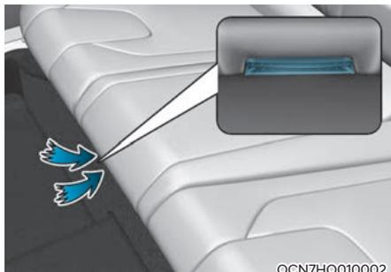
The hybrid battery cooling duct is located on the middle side of the rear seats. The cooling duct cools down the hybrid battery. When the hybrid battery cooling duct is blocked, the hybrid battery may be overheated.
