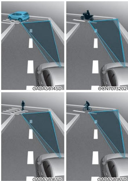
Forward Collision-Avoidance Assist may not detect other vehicles, powered two-wheelers, pedestrians or cyclists in front of you when driving on curved roads that adversely affect the performance of the sensors. This may result in no warning or braking assist when necessary.
