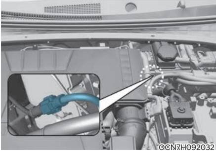
Disconnect the 12 V auxiliary battery connector located inside the engine room compartment to shut down the power of the 12 V auxiliary battery.
