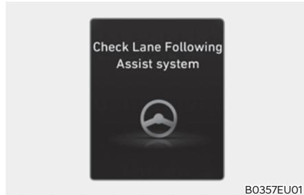
When Lane Following Assist is not working properly, the "Check Lane Following Assist system" message may appear, and the
