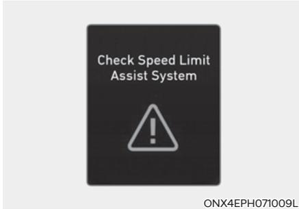
When Intelligent Speed Limit Assist is not working properly, the "Check Speed Limit Assist System" warning message may appear, and the (⚠) warning light may illuminate on the instrument cluster. Have the vehicle inspected by an authorized HYUNDAI dealer.
