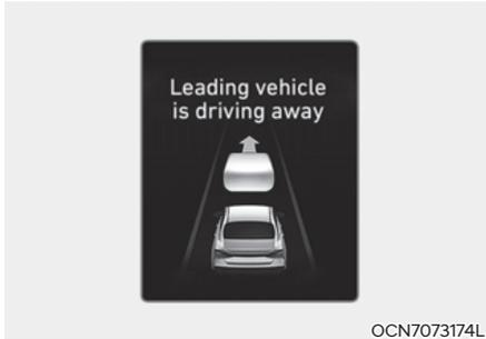
When a detected vehicle in front departs from a stop, Leading Vehicle Departure Alert will inform the driver by displaying the 'Leading vehicle is driving away' message on the cluster and an audible warning will sound.
