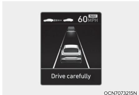
The "Drive carefully" warning message appears if Navigation-based Smart Cruise Control is not able to slow down your vehicle.
