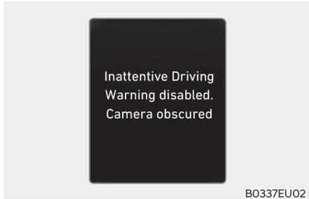
When the front windshield where the front view camera is located is covered with foreign material, such as snow or rain, it can reduce the detecting performance and temporarily limit or disable Driver Attention Warning. If this occurs, the "Inattentive Driving Warning disabled. Camera obscured" warning message will appear on the instrument cluster. Driver Attention Warning will operate properly when snow, rain or foreign material is removed.
