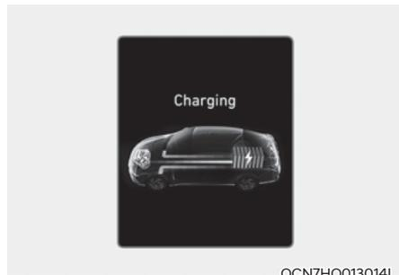
The engine charges up the high-voltage battery. The motor power is used to drive the vehicle.
