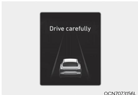
When the vehicle is stopped due to emergency braking, the 'Drive carefully' warning message will appear on the instrument cluster. For your safety, the driver should depress the brake pedal immediately and check the surroundings.
