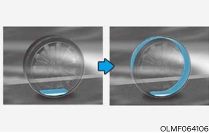
9. Immediately drive approximately 4–6 mi. (7–10 km or, about 10min) to evenly distribute the sealant in the tire.
