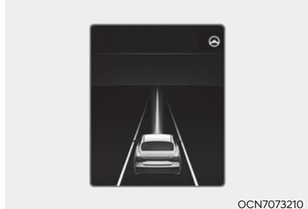
If the vehicle ahead and/or both lane markings are detected and your vehicle speed is below 120 mph (200 km/h), the green
