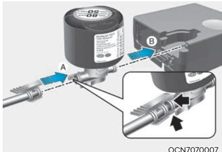
2. Connect the filling hose (3) to the sealant bottle (2) in the direction of (A) and connect the sealant bottle to the sealant bottle holder (5) in the direction of (B).
