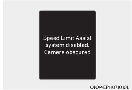
If the front view camera is covered or blocked, its detecting performance is reduced, and Intelligent Speed Limit Assist is temporarily limited or disabled. The "Speed Limit Assist system disabled. Camera obscured" warning message may appear on the instrument cluster.
