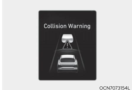
To warn the driver of a collision, Forward Safety warning light (🚦) blinking, the 'Collision warning!' warning message will appear on the instrument cluster, an audible warning will sound.
