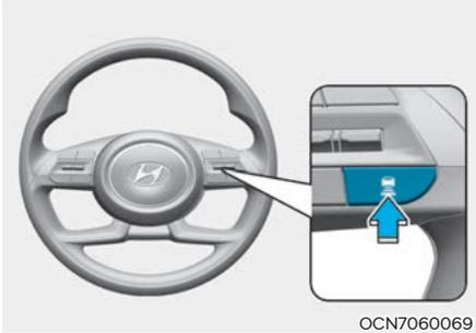
Each time the button is pressed, the vehicle distance changes as follows:
