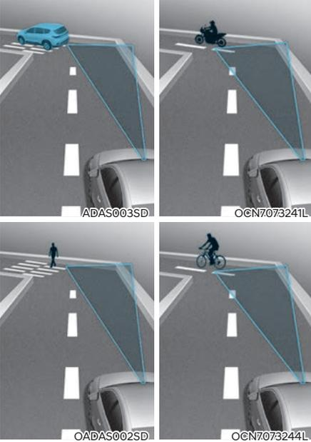
Forward Collision-Avoidance Assist may not detect other vehicles, powered two-wheeler, pedestrians or cyclists in front of you when driving on curved roads adversely affecting the performance of the sensors. This may result in no warning or braking assist when necessary.
