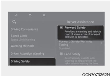
With the ignition switch ON, go to **User Settings > Driver Assistance > Driving Safety** from the settings menu in the instrument cluster or **Setup > Vehicle > Driver Assistance > Driving Safety** from the settings menu in the infotainment system to select the following:
