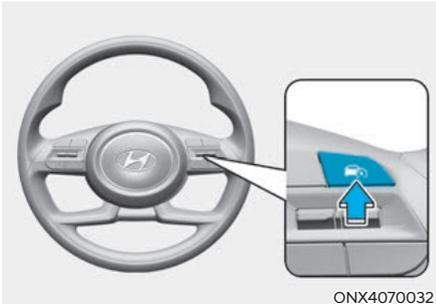
1. Press and hold the Driving Assist (
