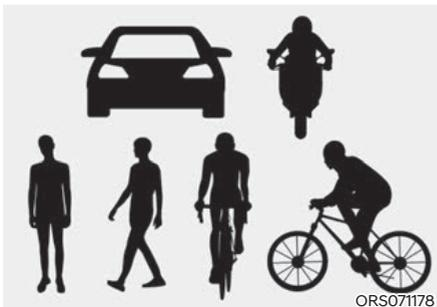
The illustration above shows the image the front view camera is capable of detecting as a vehicle, powered two wheeler, pedestrian and cyclist.
