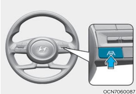
With the ignition switch ON, press the Lane Driving Assist button on the steering wheel to turn on Lane Following Assist. The white or green
