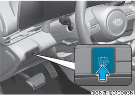
7. Press the 12 V Battery Reset switch.
