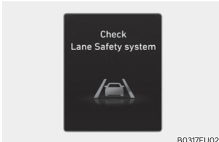
When Lane Keeping Assist is not working properly, the 'Check Lane Keeping Assist (LKA) system' warning message will appear and the yellow
