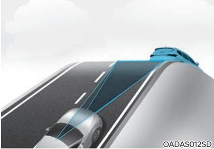
During uphill or downhill driving, Smart Cruise Control may not detect a moving vehicle in your lane, and cause your vehicle to accelerate to the set speed. Also, vehicle speed will rapidly decrease when the vehicle ahead is detected suddenly.
