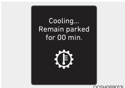
If you move the vehicle to a safe location and shift the gear to P (Park) with the engine running, the above warning message appears.
