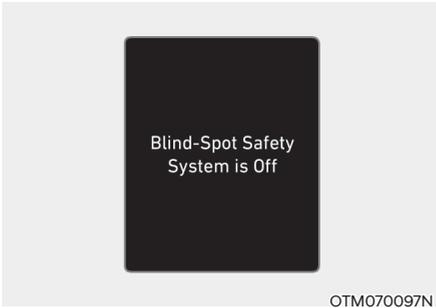
When the engine is restarted with Blind-Spot Collision-Avoidance Assist off, the 'Blind-Spot Safety System is Off' message will appear on the instrument cluster.
