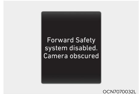
When the front windshield where the front view camera is located or the sensor is covered with foreign, such as snow or rain, it can reduce the detecting performance and temporarily limit or disable Forward Collision-Avoidance Assist.
