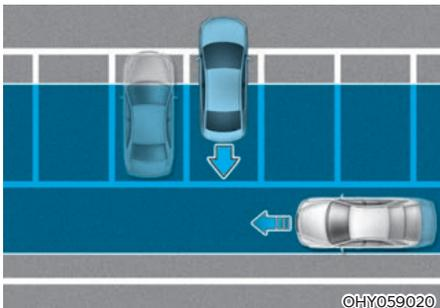
Rear Cross-Traffic Collision-Avoidance Assist may detect vehicles passing by behind you when parking backwards into a parking space. If this occurs, the system may unnecessarily warn the driver and control the brake.
