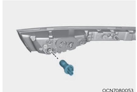
5. Remove the socket from the assembly by turning the socket counterclockwise until the tabs on the socket align with the slots on the assembly.
