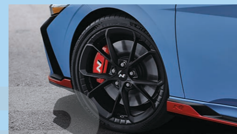
19" forged wheels and 14.2" front brake rotors
